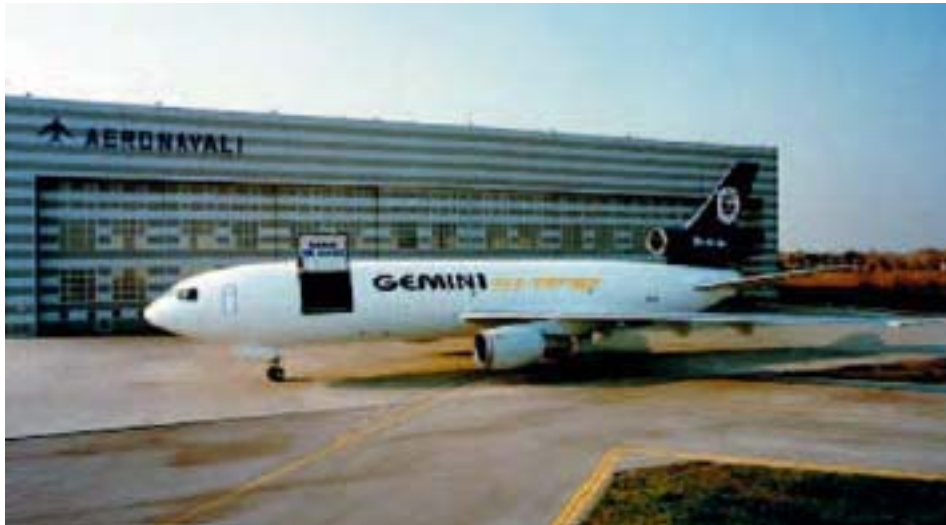
US-based Gemini Air Cargo operates MD-10 freighter converted by Aeronavali.
