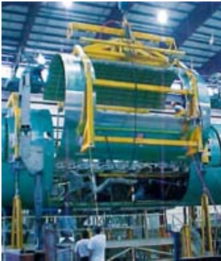
Installation of large cargo door on B757-200.
