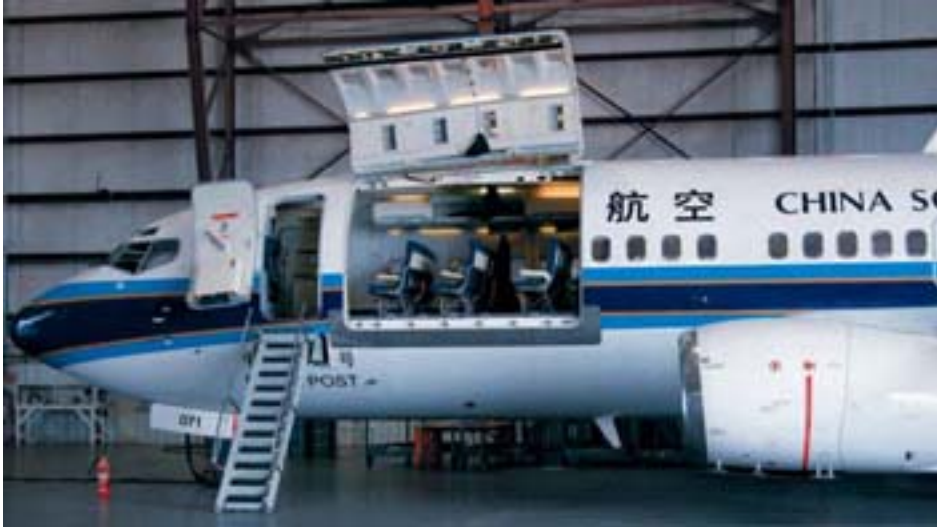
Pemco's conversion of 737-300-400s include China Southern 737QC operated by China Post.
